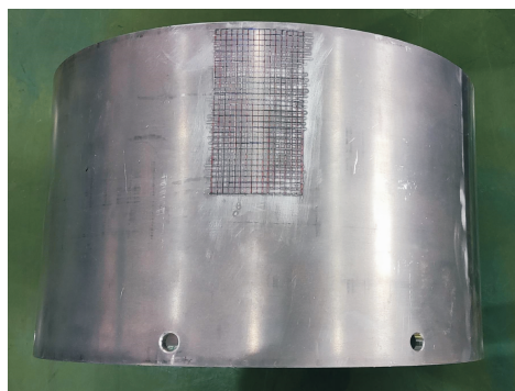
(b)卷焊筒体坯料实物
